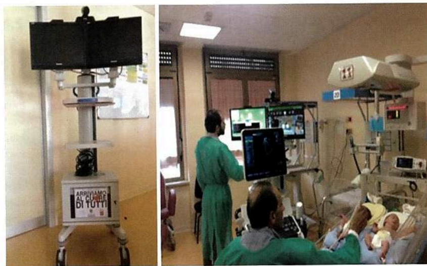
Fig. 16.7 The telemedicine cart (on the left) was set up in neonatology at Arezzo Hospital including the following: videoconference equipment is connected with digital video output of echocardiography instrumentation (on the right); two monitors are provided: one for videoconferencing and the other for medical reporting. All inputs are medically insulated
